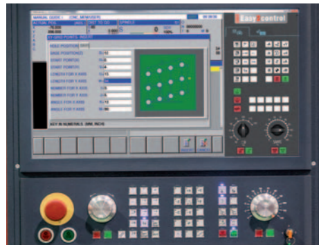
The change to a different control system is carried out within a minute by calling up the respective software
