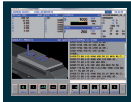
WinNC for Fanuc 31i-B including Manual Guide i is one of the WinNc controls.
